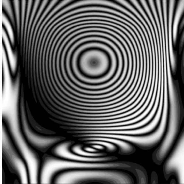
Figure 4. Isoclinics and isochromatics intertwined (the image produced by the plane polariscope) with smoothing for the sixth eigenmode at  $\alpha = 3\pi/8$ .
