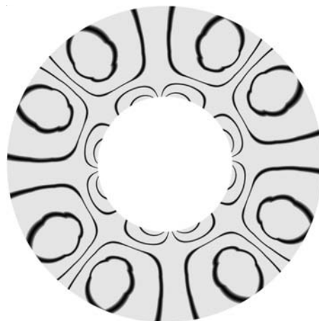
Fig. 3. Composite isoclinic pattern for the values of \alpha = (i-1)\pi/20 , where i = 1, \dots, 10
