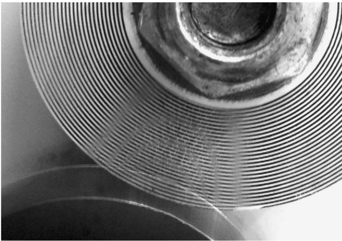
Fig. 7. Time-average photograph of the vibrating rubber roller.
