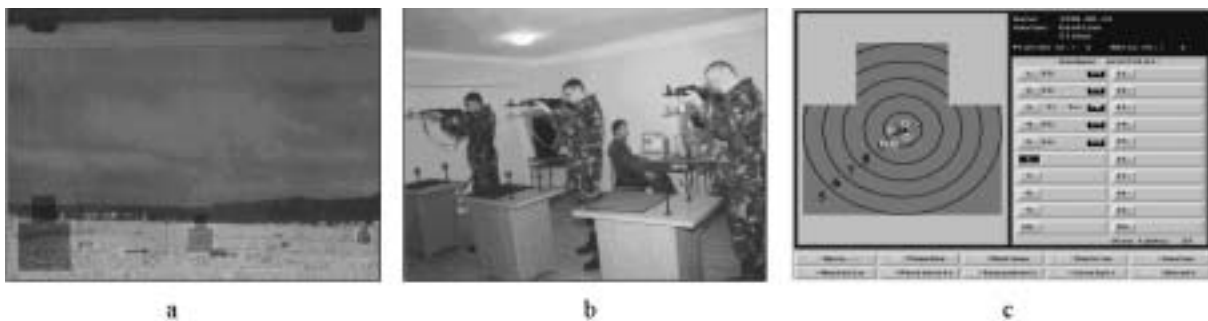
Fig. 9. Laser rifle trainer LT-2: a – multimedia target view on the screen; b – fire line and working place of instructor; c – information on monitor.
